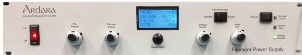
Figure 1. Front Panel Controls for Filament Power Supply
