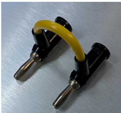
Figure 4. Example of one of the Jumpers that are used to shunt out one of the inductor coils.
